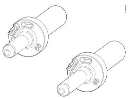
Plungers can be easily changed. Refer to the *Figure: Plunger change*. Press the plunger and rotate and align the groove on the plunger to the pad on the body of the tool. Remove the plunger and make the opposite process with suitable plunger.
