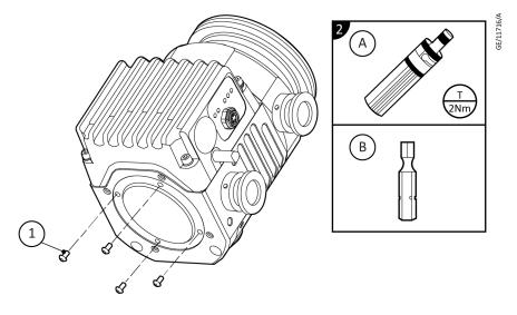
A. Tool - Torque screwdriver
