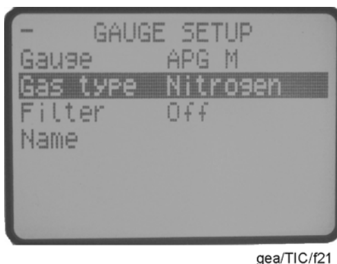
Figure 18 - Gauge setup screen
