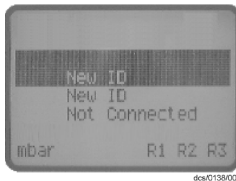
Figure 16 - New gauge connected
