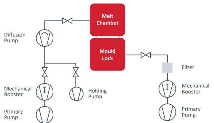
Typical layout for PIC operation
