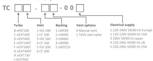
nEXT730/930 variants cannot be used with 110-120V 50/60 Hz USA voltage Important note: System is not UL certified.
